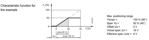
The effective span  $\Delta Uw = 10 \text{ V}$  - Uo is between 0 V and 10 V
