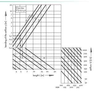
$\Delta$  12 at warm air supply, is positive, and at cold air supply, is negative. The deflection of the stream Y is directed upwards for a warm supply air and downwards for a cold supply air.
